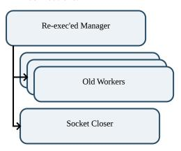
3. Manager process re-execs itself. It picks up new configuration and code while maintaining the same PID as the old manager process. At this point only the socket-closer is tracking the old workers, but everything (including old workers) remains a child of the new manager process. As a result, old workers are *not* discoverable with swift-orphans; swift-oldies may be useful, but will also find the manager process.
