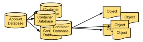
To keep track of object data locations, each account in the system has a database that references all of its containers, and each container database references each object.
