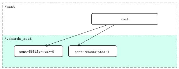
Each shard container has an *own\_shard\_range* record which has the lower and upper bounds of the object namespace for which it is responsible, and a reference to the sharding user container, which is referred to as the *root\_container*. Unlike the *root\_container*, the shard containers *own\_shard\_range* does not cover the entire namepsace.
