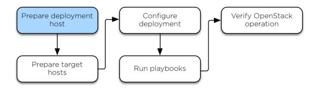
When you install OpenStack in a production environment, we recommend using a separate deployment host that contains Ansible and orchestrates the OpenStack-Ansible (OSA) installation on the target hosts. In a test environment, we recommend using one of the infrastructure target hosts as the deployment host.
