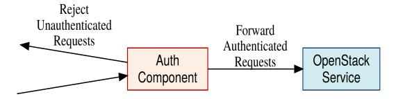
The Authentication Component, or middleware, will reject any unauthenticated requests, only allowing authenticated requests through to the OpenStack service.
