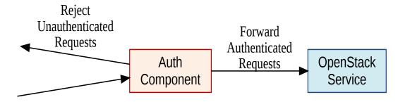
The Authentication Component, or middleware, will reject any unauthenticated requests, only allowing authenticated requests through to the OpenStack service.
