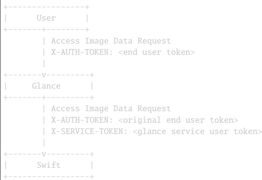
When a service receives a call from another service, it validates that the token has the appropriate roles for a service user. This is configured in each individual service configuration, under the section `[keystone_auth_token]`.
